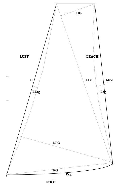
NOTE: When measuring a triangular genoa where HG = 0, LG1 and LG2 will be equal
