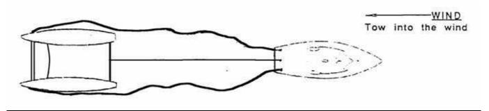
The following diagram is a section illustrating the first stage of righting a catamaran or trimaran.
