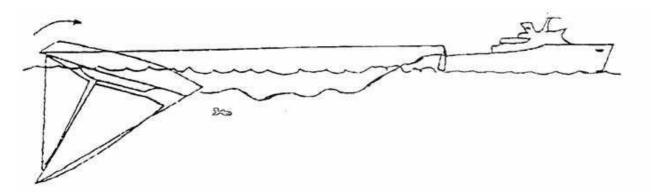
Once the yacht's stern starts to bury release the tension on the stern line and transfer the load completely to the two bow lines. However, ensure that these lines are clear and not trapped under the hulls.
